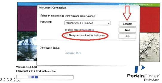
8.2.4. Make sure the Instrument being used is selected and then click "Connect".
